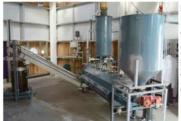
Pilot-scale biochar production facility (above) at the new purpose-built UK Biochar Research Centre (pictured right)
