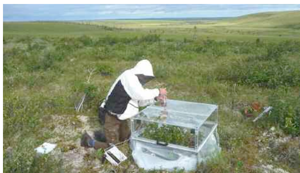
Opposite: Rut Domenech Jordi and Sophie Philbrick collecting samples from a gas flux chamber to determine soil CO 2 and CH 4 flux rates.
